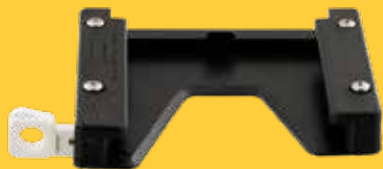
1010 QUICK-SLIDE DECK MOUNTING BRACKET Works with the 1025 through 1029 optional mounts. Dimensions: 4 ¾" x 5 ⅝" Bolting Dimensions: 2 ⅝" x 4 ⅞"
