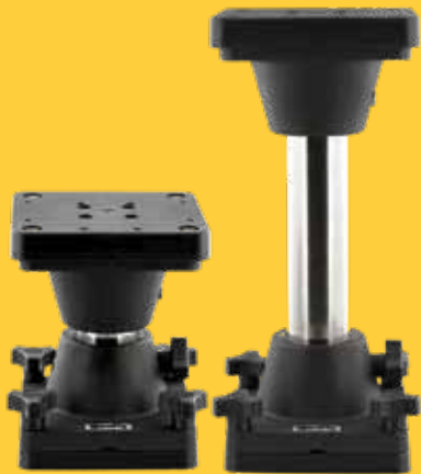
2606/2612 PEDESTAL RISER - 6" PEDESTAL RISER - 12" Made from 2" stainless steel tubing for the ultimate in strength and durability. Designed to be used with 1026 Swivel Mount., 1023 tilt-up Downrigger mount and 1010 compact Downrigger mount. Plate Dimensions: 5 ½" x 5 ½" Bolting Dimensions: 3 ½" x 4 ½"
