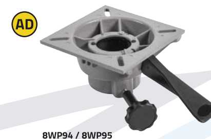
8WP94 SEAT MOUNT SPIDER Features Cast Aluminum Construction Fits 2 7/8" O.D. Pedestals Adjustment Knob Locks Seat into Place or Allows 360° Swivel Motion 8WP95 Fits 2 3/8" O.D. Pedestal
